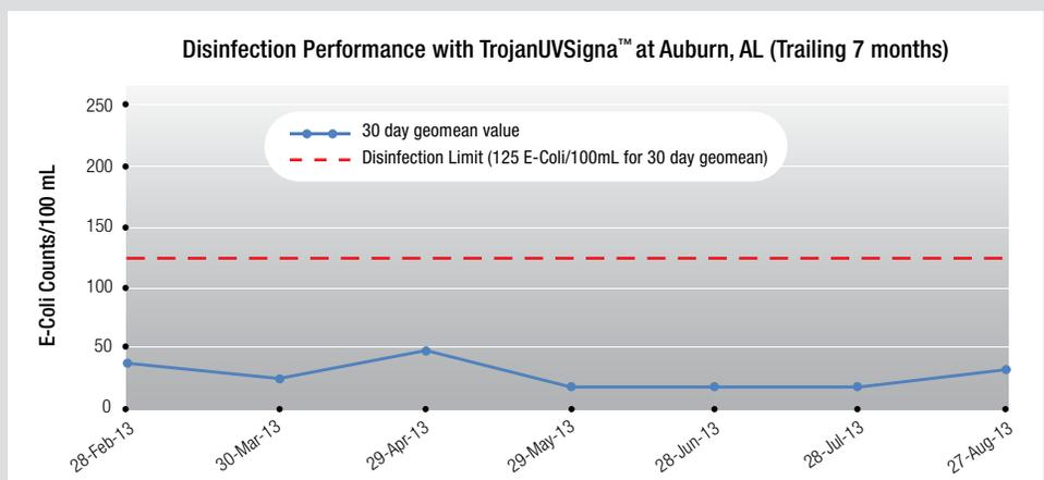
**Figure 1.** The disinfection performance of the TrojanUVSigna has consistently been below the regulatory limit for the plant.
