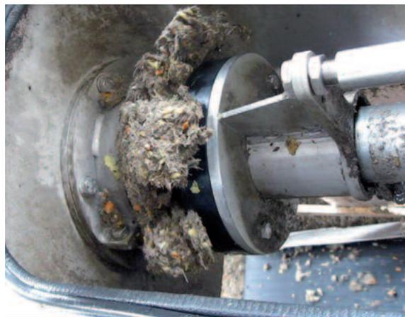
*Discharge of the separated pressed material*
