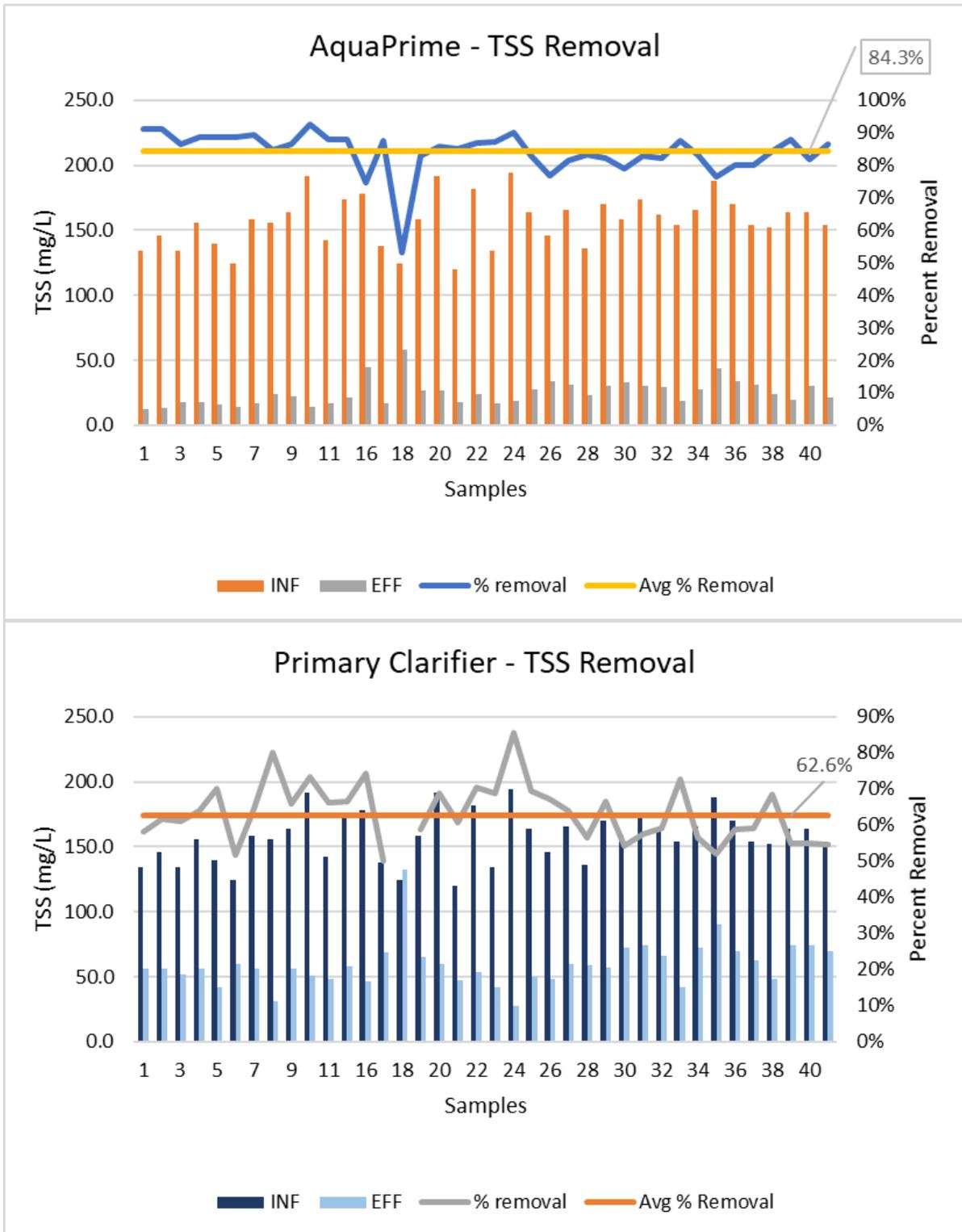
Figure 6: TSS Removal with AquaPrime in comparison to Primary Clarifiers
