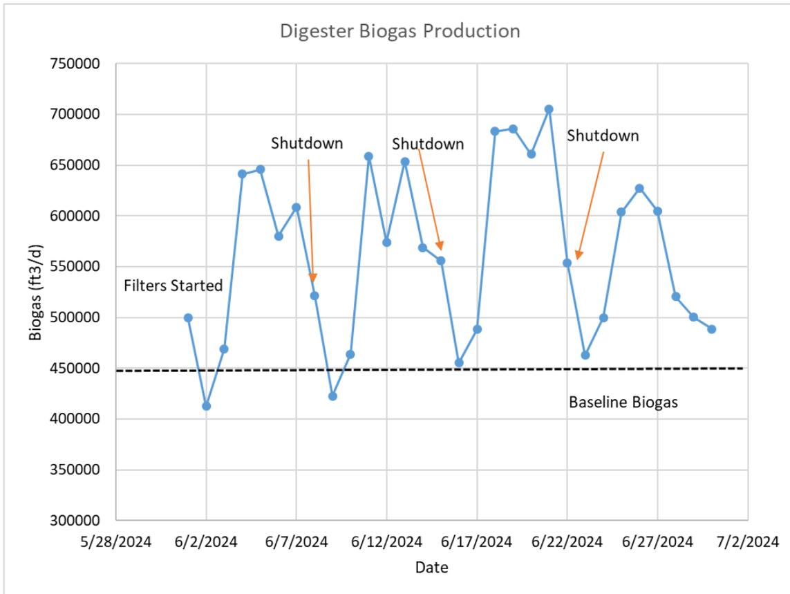
Figure 8: Digester Biogas Production after AquaPrime filters startup
