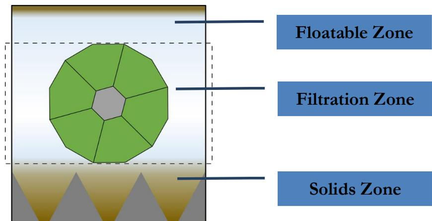
Figure 1: AquaPrime® Filter - Solids Removal Illustration
