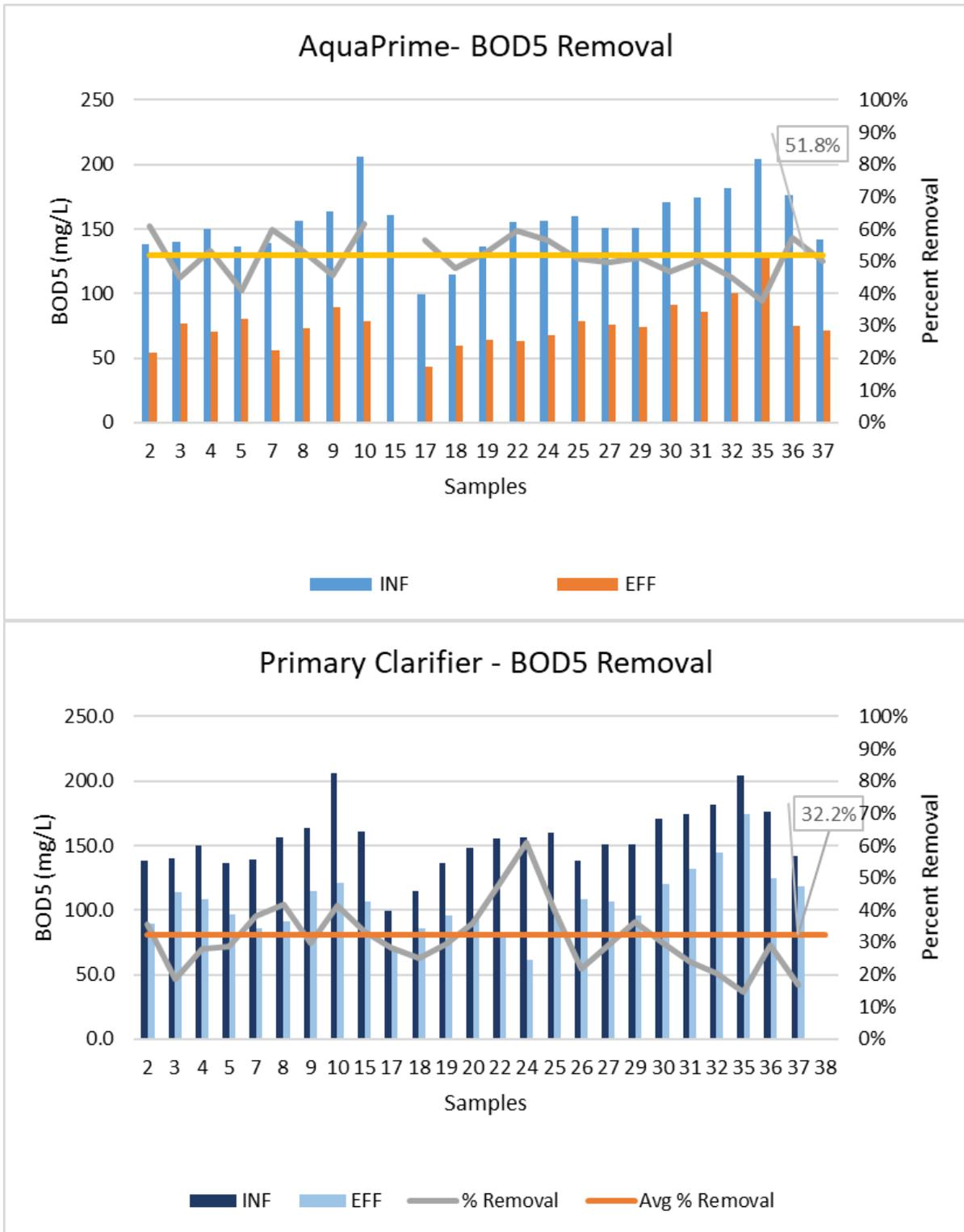
Figure 7: BOD Removal with AquaPrime in comparison to Primary Clarifiers
